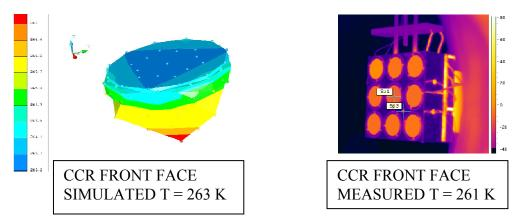
*Figure 3*: Comparison of the steady state CCR temperature measured with the SCF (ES only) and modelled with the thermal software, in a specific test configuration.
