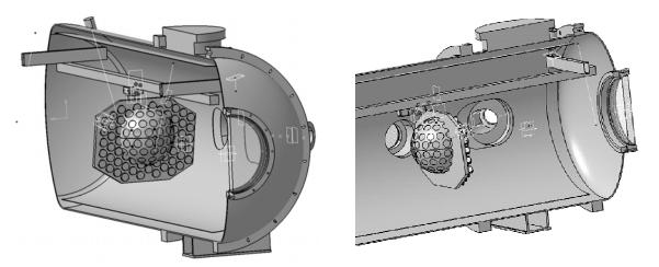
*Figure 10: The baseline LARES and a GNSS retro-reflector* array in the upgraded SCF.
