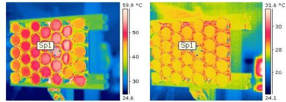
*Figure 6*: Warmest and coolest conditions of the GPS3 retro-reflectors in the LNF STP test.
