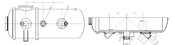
Figure 9: Left/central/right windows: IR thermometry, FFDPs and a spare.
