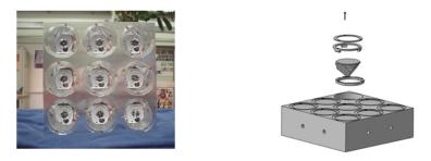
Figure 2: The 3×3 LAGEOS matrix built at LNF and the CCR assembly components.
